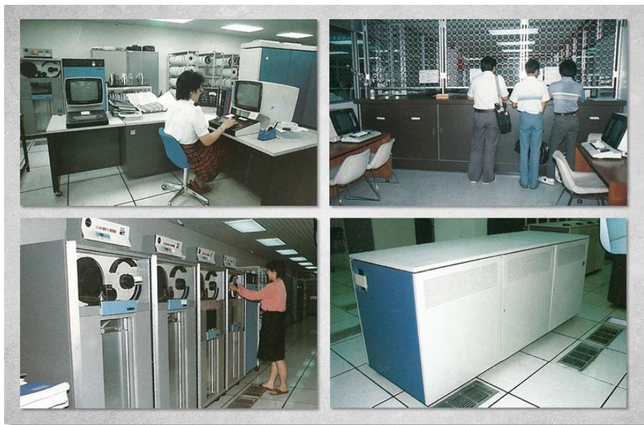
Clockwise from top: 1. the School’s supercomputers, 2. computer printout queue, 3. 1.5 MIPS processor and 4. magnetic loading disks.
